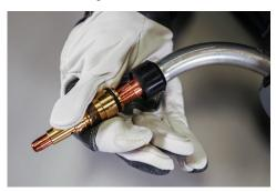
D. Remove the power pin cap from the rear of the gun
