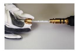
E. Place torque wrench on the power pin cap and torque to specification.
