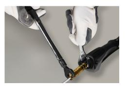
**STEP 4**Trim the liner flush with the power pin.
