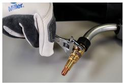
C. Remove the gas diffuser.
