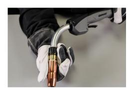
C. Identify the power pin to determine the appropriate power pin cap torque specification.
