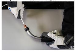
C. With the gun laying straight, push the liner through until the brass liner lock bottoms on the neck.
