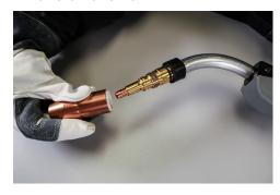
B. Loosen the gas diffuser.
