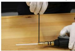
B. Insert a piece of welding wire into the liner to check for burrs or obstructions. If needed, loosen screw slightly until wire slides freely.
