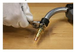
D. Loosen the set screw in the power pin cap and remove the cap from the rear of the gun.
