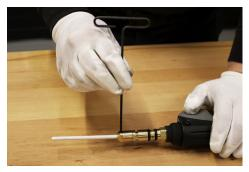
**STEP 4**A. Trim the liner flush with the power pin.
