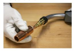
C. Remove the gas diffuser.
