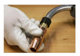
D. Tighten the cap snug against the power pin shoulder with welding pliers or appropriate wrench.
