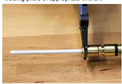
F. Next, hold the hex wrench by the handle and tighten the set screw an additional one-half turn to fully secure the liner.
