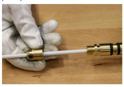
E. Holding the hex wrench as shown, tighten the set screw "finger tight" against the liner.
