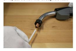
C. With the gun laying straight, push the liner through until the brass liner lock bottoms on the neck.
