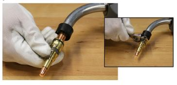
C. Place the power pin cap over the liner and thread onto power pin.
