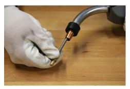
B. Loosen the gas diffuser.
