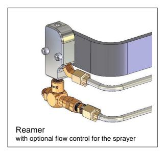
**NOTE:** Choosing Reamer option 'C' - Flow Control adds an adjustable check valve, giving users the ability to control the amount of TOUGH GARD Anti-Spatter applied in each spray. **Also available: the retrofitable flow control kit (Part #SR-500-55).**
