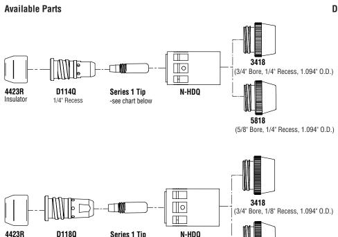
Diffusers and nozzle cones and bodies are available in packages of 10, insulators in packages of 5 and contact tips in packages of 25
