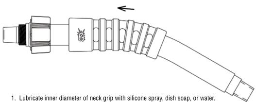
2. Install over neck armor and move to desired position. Neck grip can be used in place of rubber insulator for wrench tightened necks.
