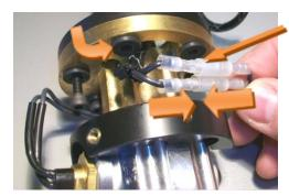
The leads from the unicable are pulled through the access hole and connected here. This connection is captured within the outer cover of the gun.
