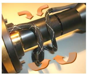
The remaining lead length from the unicable is looped, as shown to the left. The self-feeding loop will allow for rotation in both directions. This loop will be captured within the wrist of the robot.
