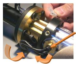
Switch leads are bent at 90° and wrapped around, as shown here.
