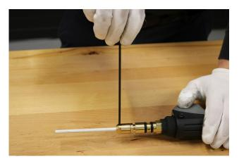
7. Insert a piece of welding wire into the liner to check for burrs or obstructions. If needed, loosen screw slightly until wire slides freely.
