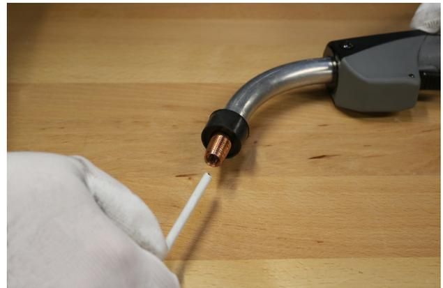
3. Lock and center liner by reinstalling the diffuser. Slide power pin cap over exposed liner and tighten the cap snug against power pin shoulder with welding pliers or appropriate wrench.
