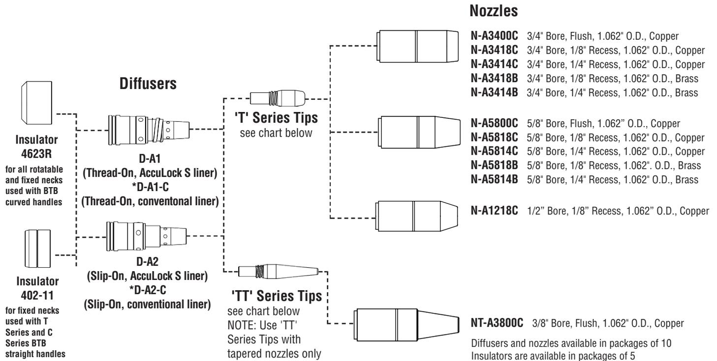
NOTE: \*Not engineered for error-proof liner replacement and flawless wire feeding. For use with Bernard conventional liners. Refer to spec sheet [SP-L](#) for more information.
