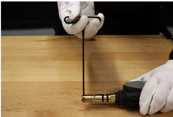
2. Replace the new liner through the neck until brass liner lock bottoms on neck.
