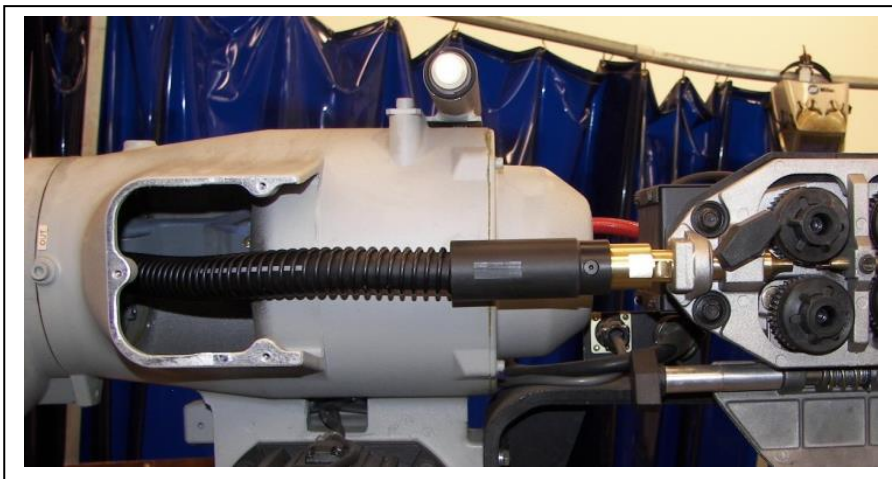
Figure 11 – Install the power pin or Euro connection to the wire feeder, as per the manufacturer's instructions. The wire feeder control cable is also added during this step.
