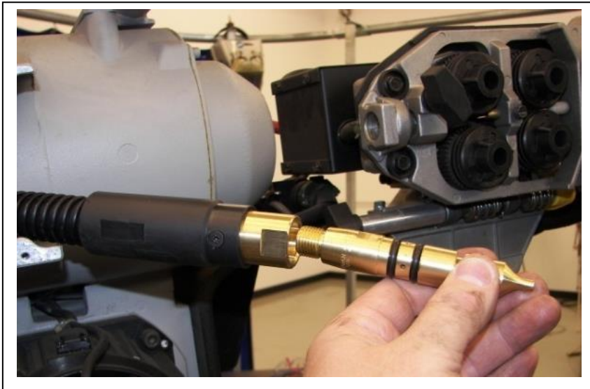
Figure 9 – Once the LSR Unicable is pulled through the robot, add the power pin (or Euro connection).
