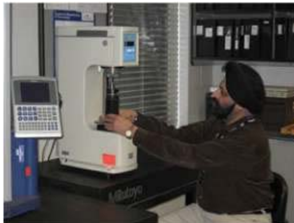
the Mitutoyo Rockwell ATK-600 hardness tester gets frequent use at quality-conscious tregaskiss.
