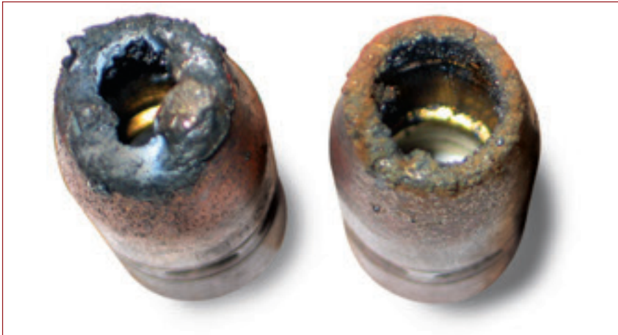
Fig. 3 — Examples of nozzle spatter buildup. Checking the nozzle periodically for spatter buildup and proper cleaning can extend the life of the consumable. Applying an antispatter product can also help prevent spatter from building up.
