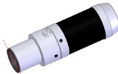
Cut liner 1/8" shorter than flush
